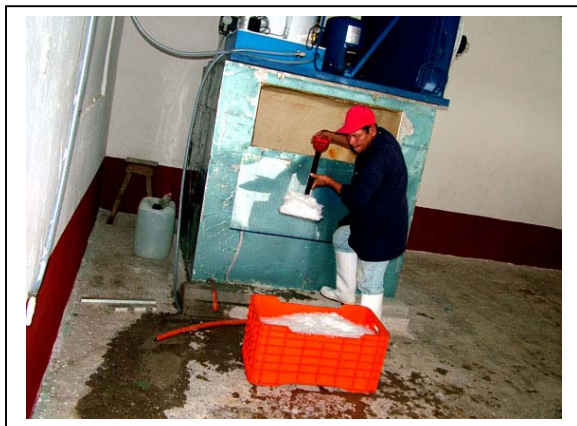
Pictures 4 and 5: the ice plant working in Tamiahua (production capacity of 2,5 MT/day) and the ice being used to refrigerate fishes in boxes also supplied by the project.
